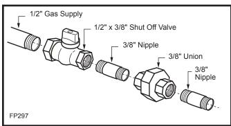
Fig. 7 Typical gas supply installation.
